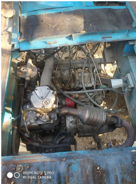
Fig.7 Diesel Engine with Gearbox
